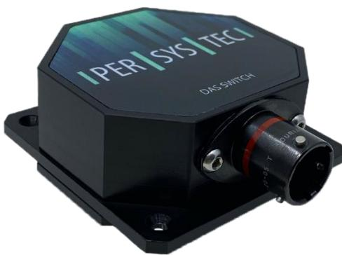
switching between 2 independent Input signals but also scaling the signals to the same output range thus a single ECU calibration can be used regardless of the sensor selection.
